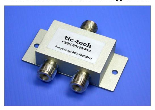
Model PS2N-80100/P10 2 way divide **Type** Frequency 800-1000MHz VSWR for full bandwidth <1.5:1 <0.5dB **Insertion Loss** Isolation >20dB 50 ohms Impedance **Input Power** 10 watts **Operating Temperature** -30°C ~ +60°C Connector **N** Female **Dimension** 90 x 72 x23 mm Weight Approx. 0.16KG
